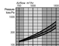
The following aspects affect the pressure loss in PlymoVent's LM-2:
